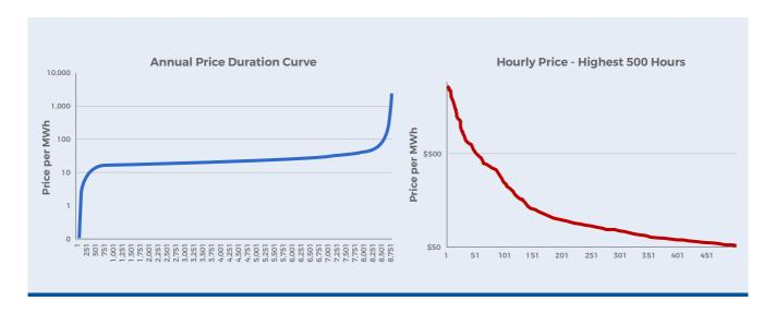
On the above chart, we see the top 500 hours of this price duration curve are above approximately \$50/MWh. Offering a unit to deploy at this price allows one a chance to fully utilize the available hours.
