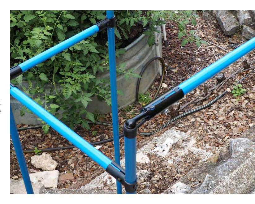
The "locking" mechanism is a rubber chair leg cap (pipe foot) with a hole drilled into it.
