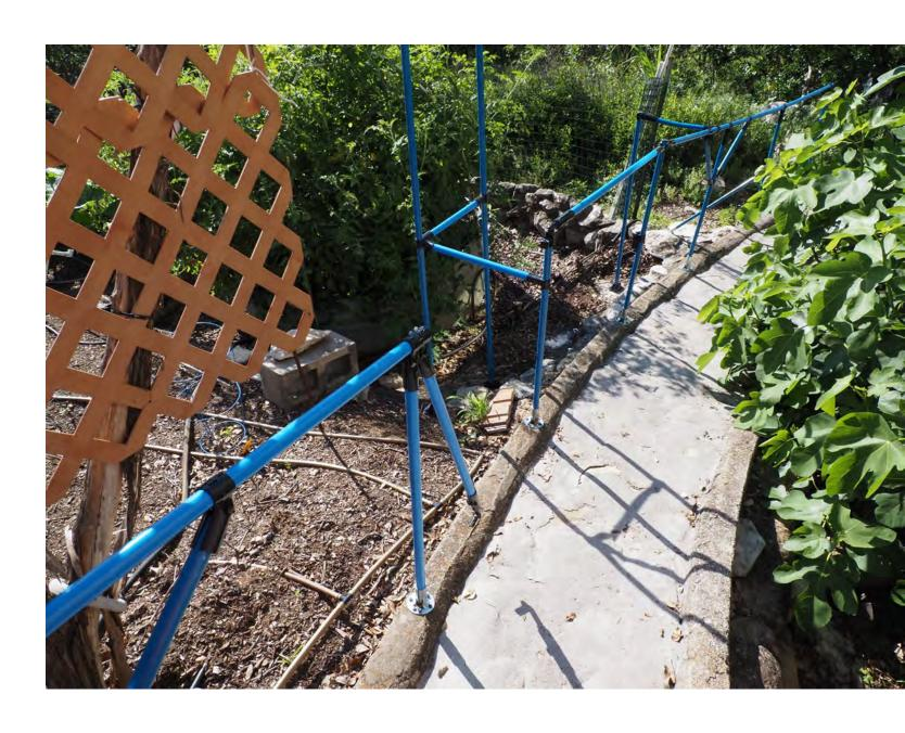
In this situation I used an adjustable angle hinge connector seen here in the closed position.
