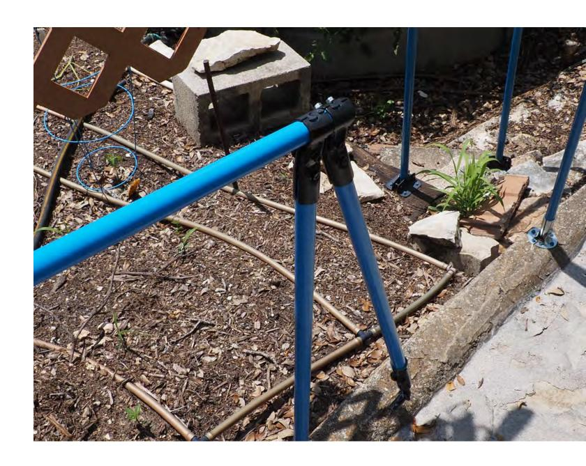
I used a lag screw post hook and lag screw hinge for the receiver.
