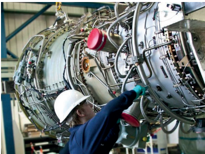
SGT-A35 (Industrial RB211) SGT-A35 gas generator maintenance, repair and overhaul
