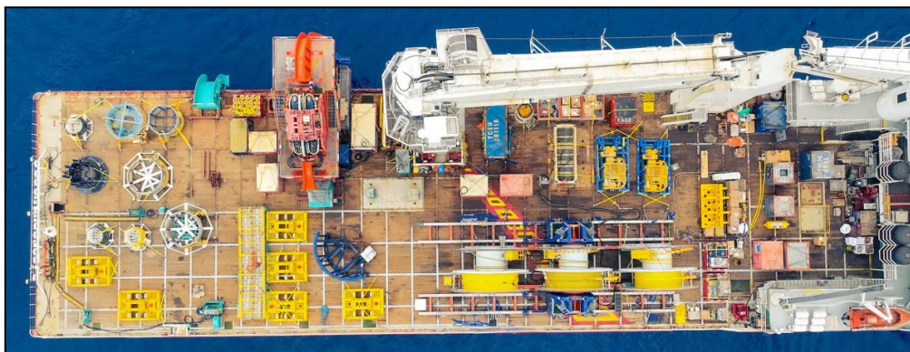
Figure 11 –Skandi Acergy Subsea construction vessel with HLS and reel drive system. Note the cable can be configured with a VLS system, as used for the base case marine spread setup.
