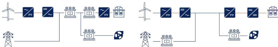
Hybrid electrical layouts with existing grid connection (left) and future connection with innovative converters (right) for a large scale green hydrogen plant with electrolyzers and e-consumers
