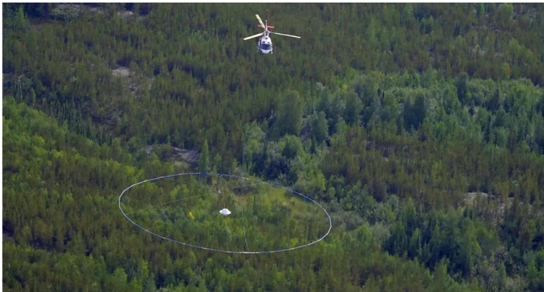
In order to survey large areas quickly, KoBold uses a helicopter carrying a transmitter coil loop 35 meters in diameter that can detect conductive bodies, such as ore deposits, below the surface.KOBOLD METALS
