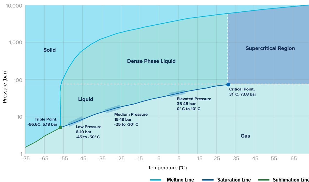
Figure 23 - CO<sub>2</sub> pressure-temperature phase diagram
