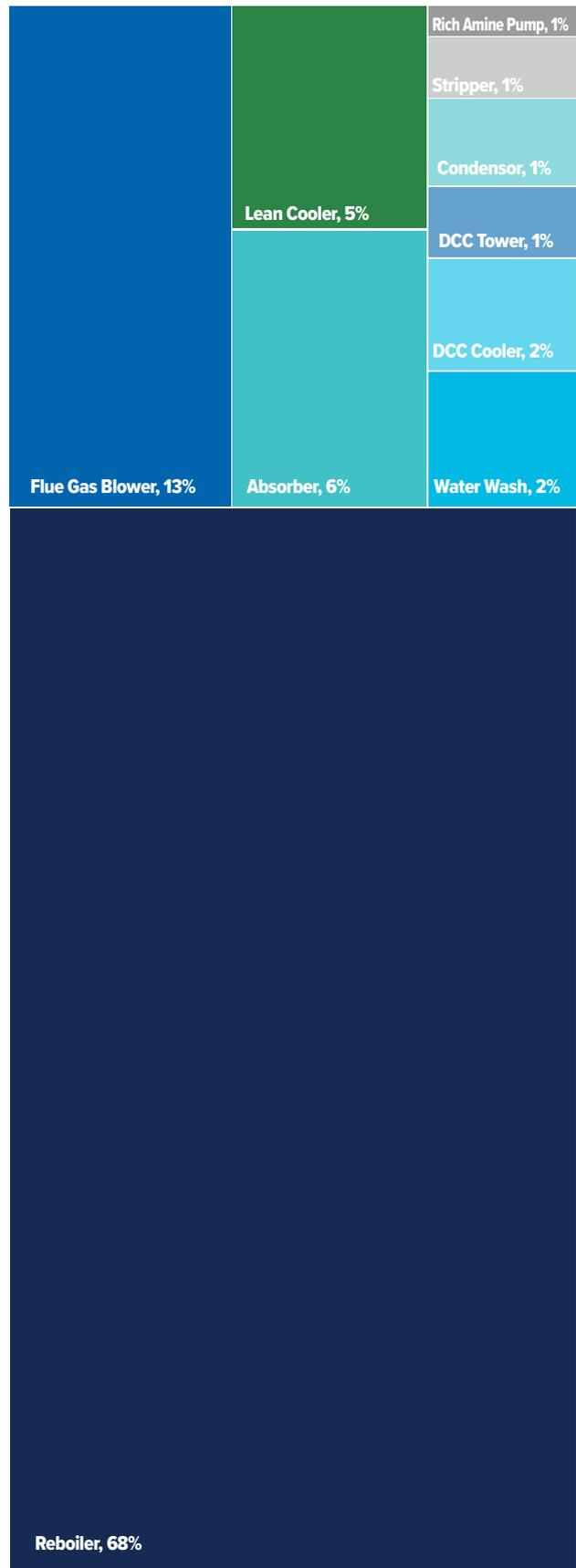
Figure 9 - Total annual costs per unit, inclusive of both capital and variable operating costs. Total Annual Costs (Capital and Operating) per Unit of the Capture Process. 90% Capture - \$77.26 US/tonne CO<sub>2</sub>
