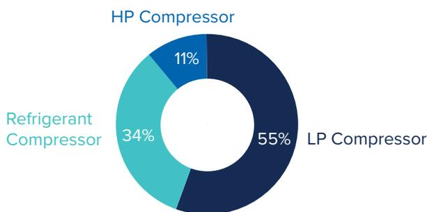
(b) Low-Pressure Liquefaction Annual Utility Cost Breakdown by Equipment
