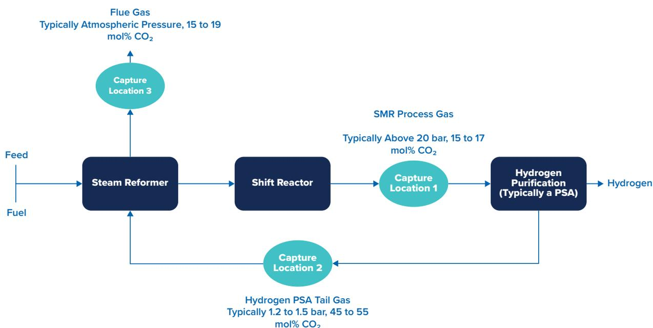
**Figure 12 - SMR hydrogen production process diagram with CO<sub>2</sub> capture locations (IEAGHG, 2017)**
