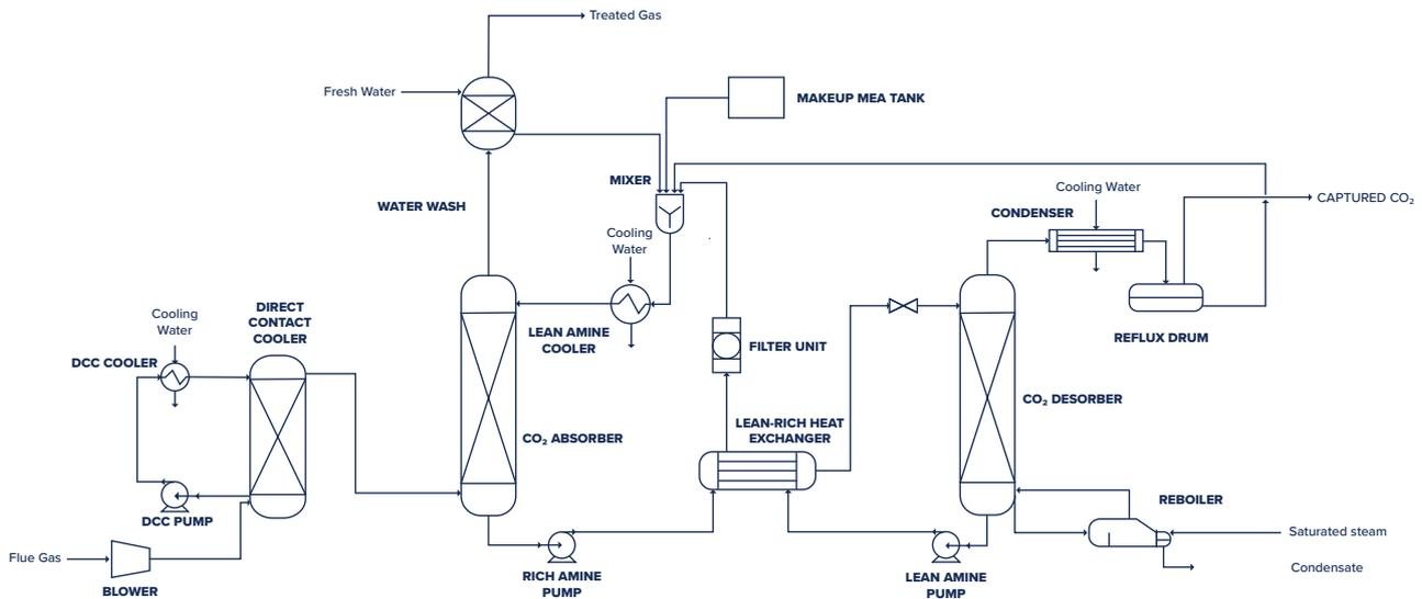
**Figure 4 - Typical MEA Capture Plant Arrangement**
