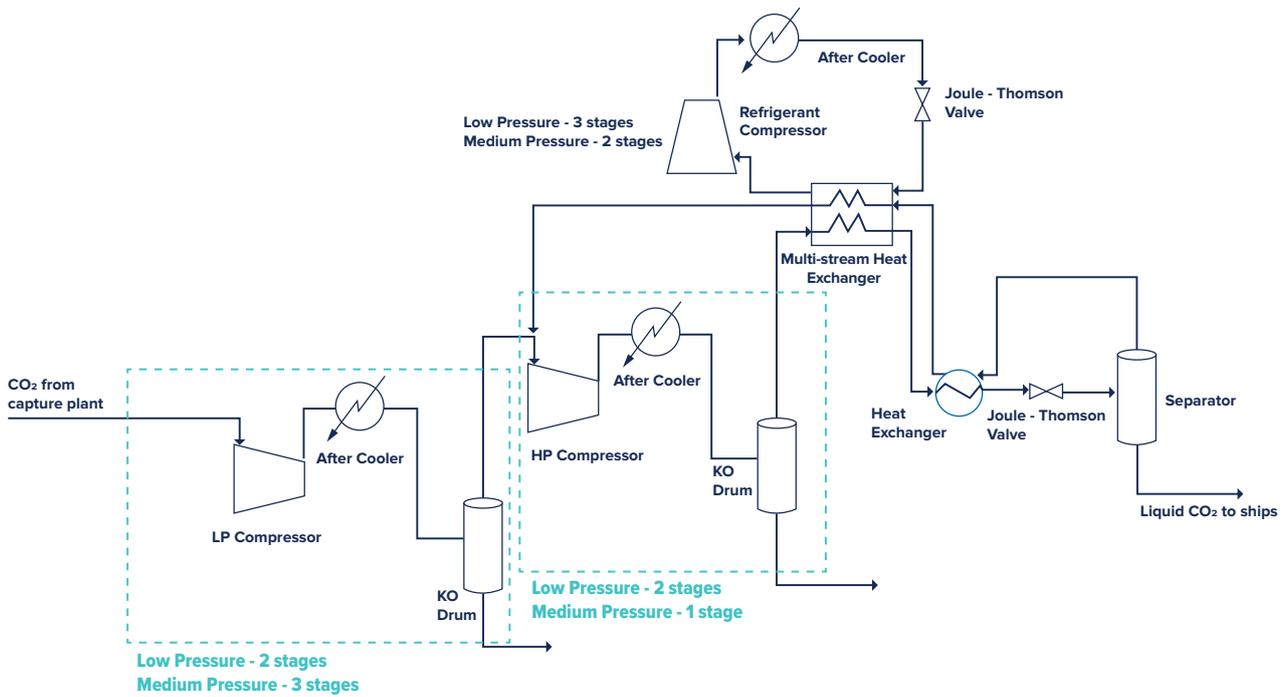
Figure 24 - Process flow diagram of CO<sub>2</sub> liquefaction (Pre-cooled Linde Hampson). (Adapted from Seo et al., 2015)
