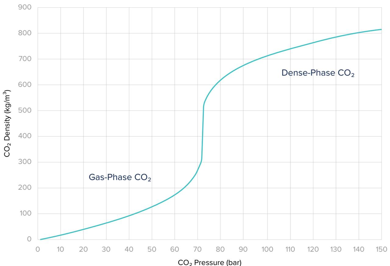
Figure 19 - CO<sub>2</sub> density at 30°C as a function of pressure
