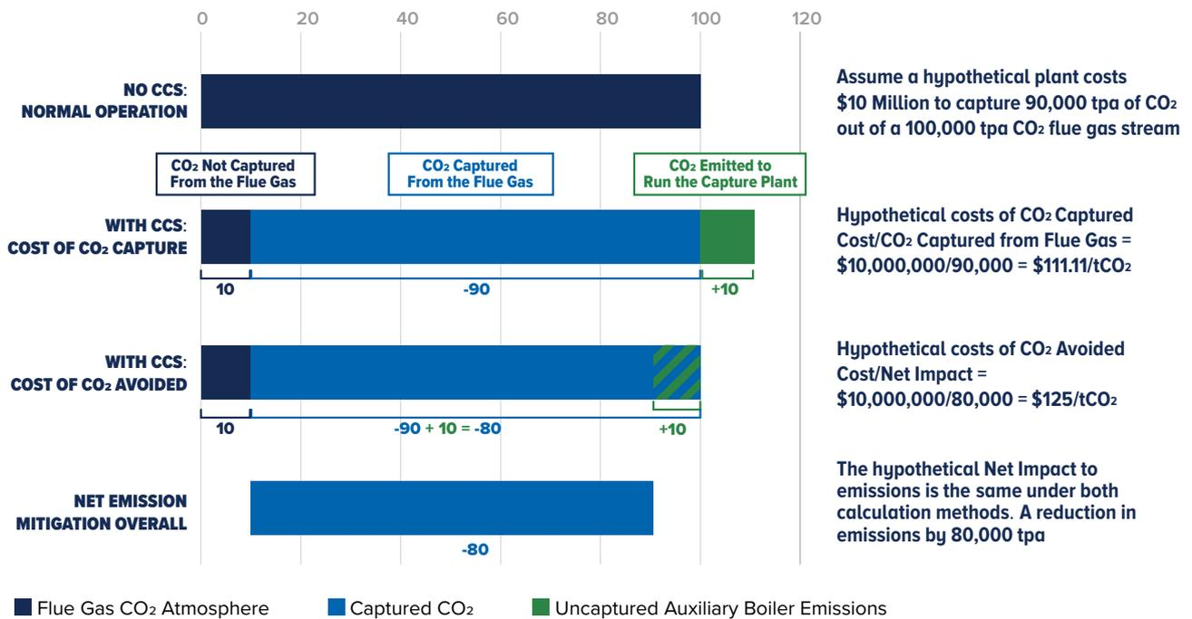
Figure 5 - Visualisation of the CO<sub>2</sub> flows and costs associated with a CO<sub>2</sub> capture plant
