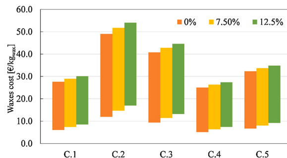
Fig. 9. Ranges of the cost of FT waxes production under different interest rates. The minimum price level corresponds to hydropower electricity source, the maximum to baseload one.
