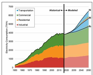
Figure 1. National demand for electricity from various sectors, three projections for future load growth based on expectation electrification of end uses such as transportation and heating. *Source: Mai et al.,* https://www.nrel.gov/docs/fy18osti/71500.pdf
