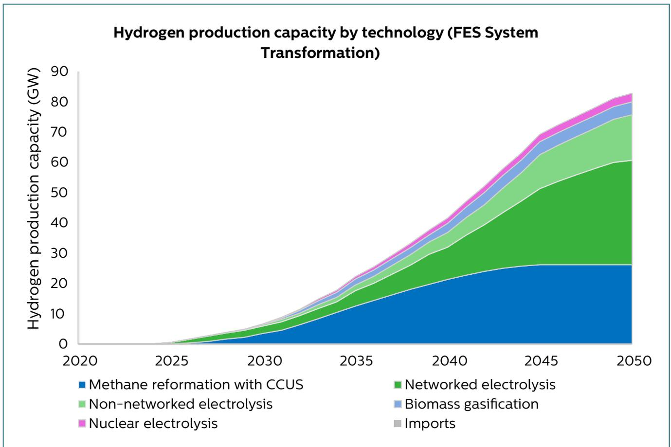
Figure 1: Hydrogen production capacity by technology (FES System Transformation)<sup>12</sup>
