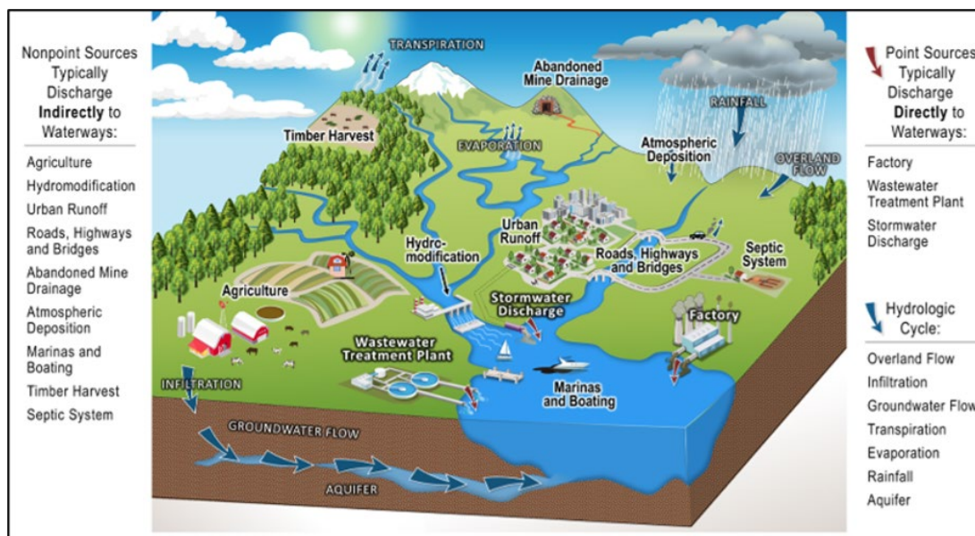
Illustrations of nonpoint and point source pollution along with elements of the hydrologic cycle
