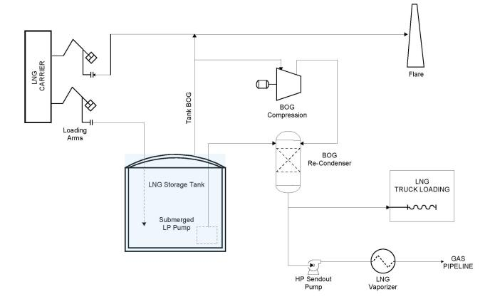
Fig. 1a LNG Import Facility Schematic
