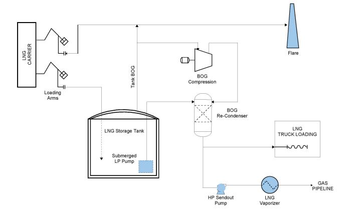
Fig. 1c LNG Import Facility Schematic
