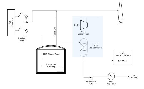
Fig. 1b LNG Import Facility Schematic
