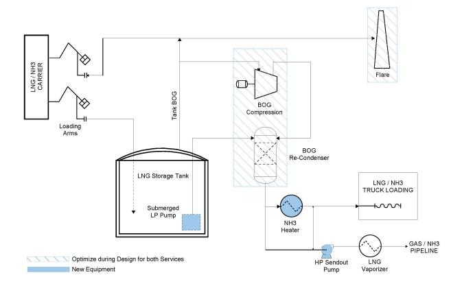
Fig. 5 Ammonia Ready LNG Import Facility Schematic
