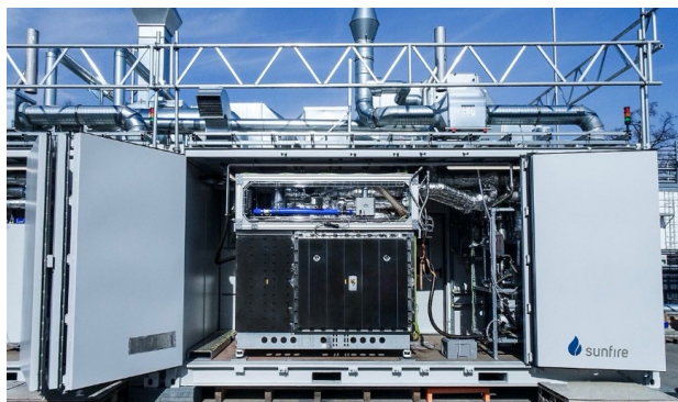
Figure 22: One of Sunfire’s SOEC Modules at the MultiPLHY Site 45
