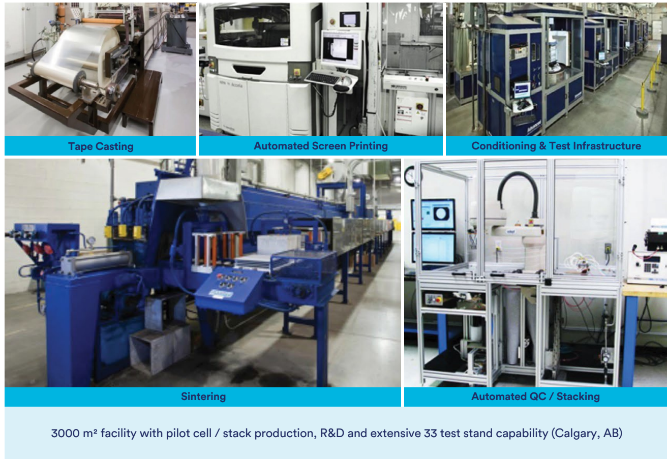
Figure 33: Solid Oxide Cell Fabrication Processes and Robots 67
