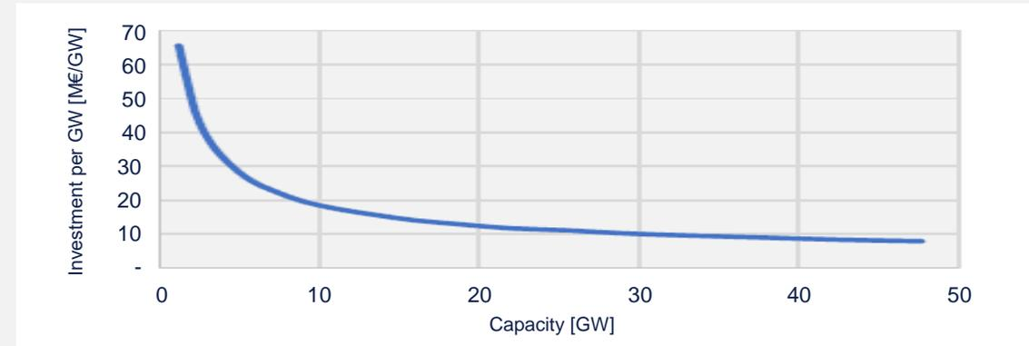
Specific investment cost for a hydrogen pipeline with increasing pipeline capacity (assumed inlet pressure: 100 barg, outlet pressure 30 barg, length 100 km). Source: DNV
