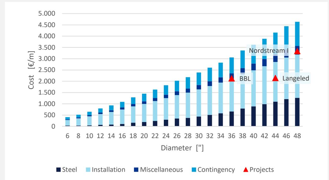
Investment figures for hydrogen pipelines depending on the diameter.
