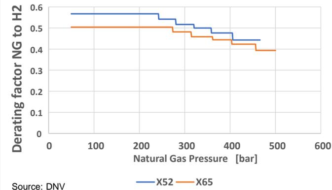
The derating factor in ASME B31.12 determines the Maximum Allowable Operating Pressure (MAOP) of the pipeline operating with hydrogen, and always results in a reduction of pressure when compared to operation with natural gas.
