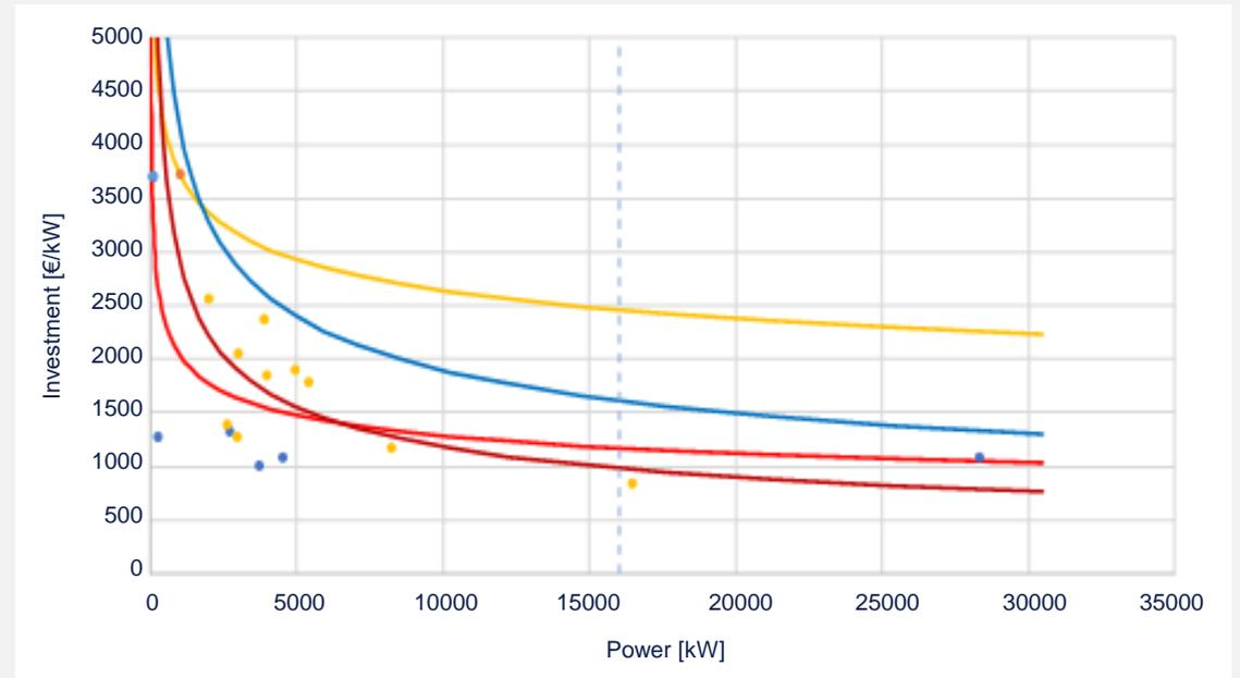
Investment figures for hydrogen compressors. Dots are individual reference prices and lines represent fitted models. Source: DNV reference database.
