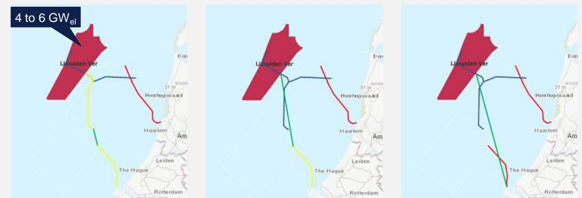
Case study for connecting IJmuiden Ver to the Maasvlakte<sup>2</sup>. The left picture is for a 400 MW<sub>el</sub> offshore electrolyser, the middle for 1 to 2 GW<sub>el</sub> (required pipeline diameter: 16", resp. 36"), the right picture is for > 2 GW<sub>el</sub>. Yellow lines are reused natural gas pipelines, green lines are newly built hydrogen pipelines. Source: DNV
