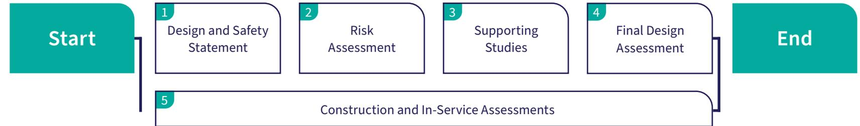
Lloyd's Register's requirements for Ships Using Methyl Alcohol (Methanol) or Ethyl Alcohol are contained within Appendix LR1 to the Rules and Regulation for the Classification of Ships Using Gases or Other Low-flashpoint Fuels, and which incorporates MSC.1/Circ.1621. These requirements follow a risk-based approach where the fundamental requirement is to demonstrate an equivalent level of safety to that achieved with conventional oil-fuelled systems.
