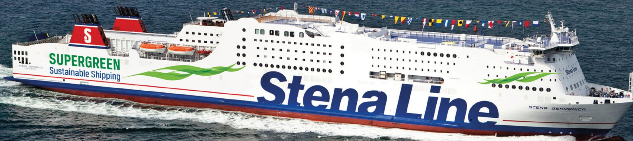
The LR-class Stena Germanica was the first conversion project demonstrating methanol fuel capabilities. Initially one of the four Wärtsilä ZS40 engines of the 2001-built vessel were converted to be dual-fuelled, capable of running off methanol or marine diesel or gasoil. Shortly after the remaining three engines were also converted to be methanol dual-fuelled. The conversion project was EU funded.
