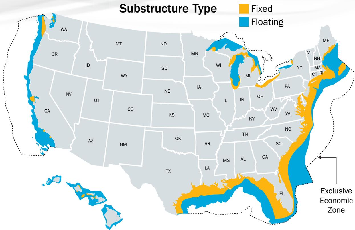
**Figure H-3** Offshore wind substructure type by water depth (60 m). Image from NREL.
