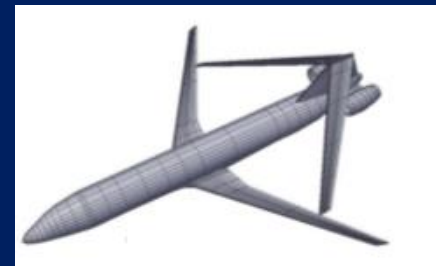
Box Wing aircraft to enable multiple fuel and engine pods while reducing drag.
