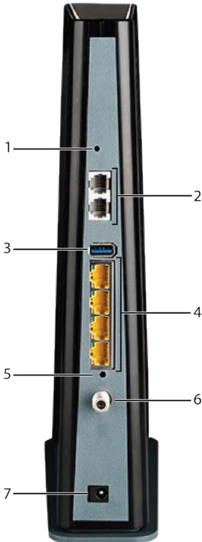
1. Connect one end of the coax cable to the cable outlet or splitter, and the other end to the Telephony Gateway's Cable connector (6). Tighten the connections by hand, then tighten an additional 1/8 turn with a wrench.
