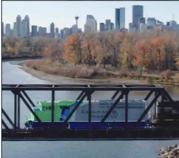
The CP Hydrogen Locomotive Program is deploying a series of **freight locomotives** into revenue service. These locomotives are powered exclusively by hydrogen fuel carried onboard, which is used by the fuel cells to generate electric traction power to haul trains. The first of these vehicles – a road switcher – was demonstrated in revenue service in Calgary in late-2022 [43].
