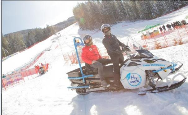
**Snowmobiles** – a feature of life in northern and remote communities – are being trialed in Austria using hydrogen fuel cells instead gasoline combustion engines for all-electric propulsion. [42]
