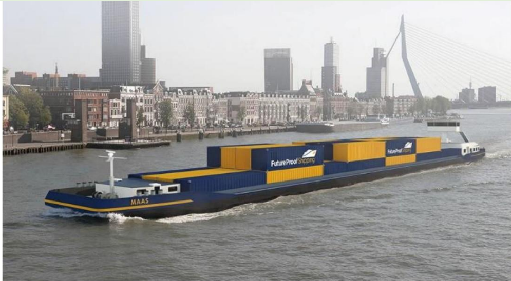
FPS Maas, retrofitted inland container vessel with 2x 500kg compressed hydrogen in swappable containers 1
