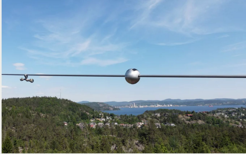
Heimdall Power's orb tracks line sag, ambient temperature, sunlight intensity, and other metrics on a transmission line in southwestern Norway. HEIMDALL POWER
