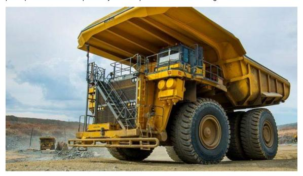
The above is an Anglo American 510 tonne<sup>22</sup> truck. It's powered by electricity, generated by eight 100 kW fuel cells, fueled by hydrogen, plus a 1.2 MW battery to store energy for peak demand.<sup>23</sup>
