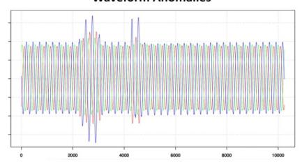
A large portion of anomalies represent normal operating conditions like a breaker closing, a capacitor bank turning on, rain hitting overhead power lines, or adjacent feeder events. These operational anomalies need to be filtered out. With analytics we can identify whether the remaining anomalies match signatures that are indicative of an impending permanent fault.
