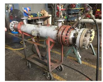
The natural gas transmitted through the pipelines is reduced in pressure from the transmission pressure (up to 700 psi) down to a pressure range of 30-50 psi for local use.
