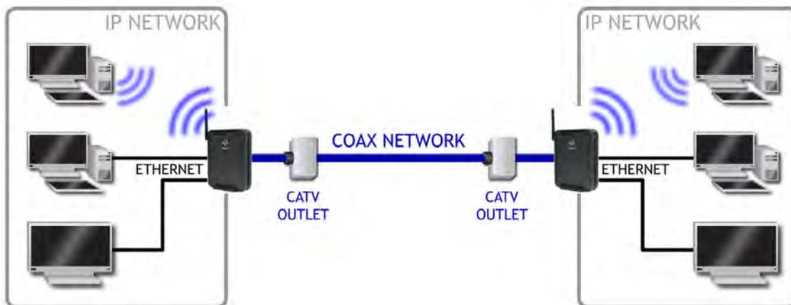
MoCA traffic on the coax network does not interfere with existing broadcasts from cable, telco, IPTV or satellite service providers, as it makes use of a previously-unused segment of the RF spectrum. The medium is ideal for real-time applications, providing high data throughput (100Mbps~1Gbps) with low latency, jitter or data loss. Also, coax cabling is generally better-shielded than IP networking media, especially wireless.
