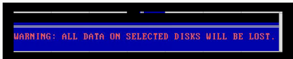
FIG. 19 Excerpt from the Remote Desktop client cache on a compromised workstation showing traces of an attempt to reconfigure the RAID array of one of the servers
