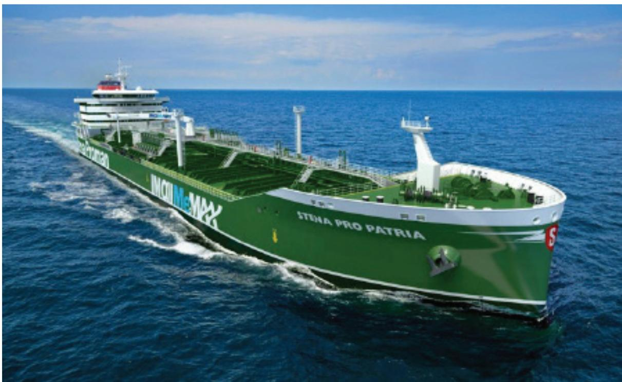
Note: Stena Pro Patria is the first of three 49,900 dwt methanol dual-fuel MR tankers by Proman Stena Bulk.
