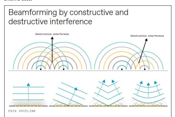
A reconfigurable intelligent surface comprises an array of unit cells. In each unit cell, a metamaterial alters the phase of an incoming radio wave, so that the resulting waves interfere with one another [above, top]. Precisely controlling the patterns of this constructive and destructive interference allows the reflected wave to be redirected [bottom], improving signal coverage.
