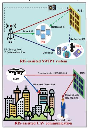
loss over long distances reduces the energy harvested at the energy receiver, which degrades the performance of SWIPT systems. However, the limitations of practical SWIPT systems can be compensated via RIS, as illustrated in In the figure to the right Through intelligent signal reflections, RIS boosts the signal strength both at the
