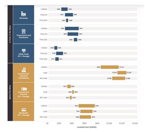
The chart below is referenced here,<sup>2</sup> and shows different configurations for a PV plus BESS. Note that the numbers are a year older than the Lizard numbers, and that these are engineering, procurement and construction (EPC) costs not LCOE.
