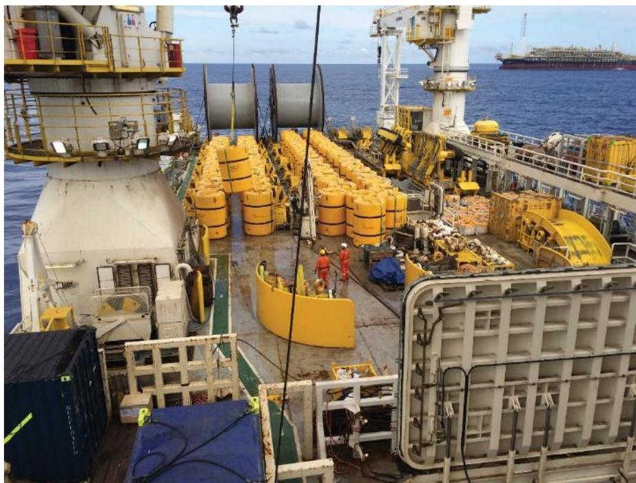
**Figure 20 Buoyancy modules stored on a vessel prior to installation.**
