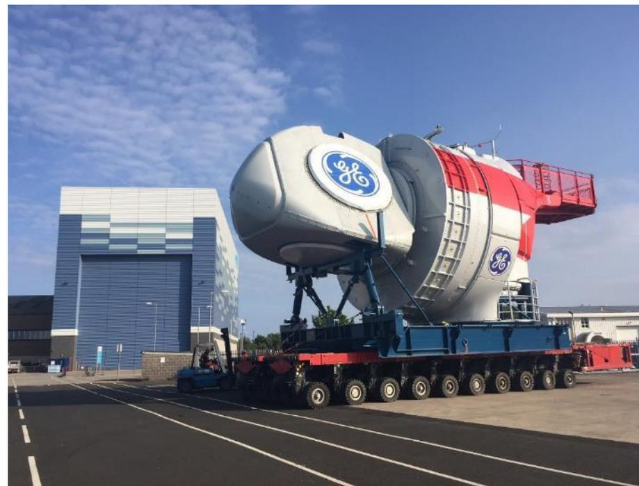
**Figure 12 GE's Haliade X 12 MW nacelle. Image courtesy of GE Renewable Energy. All rights reserved.**
