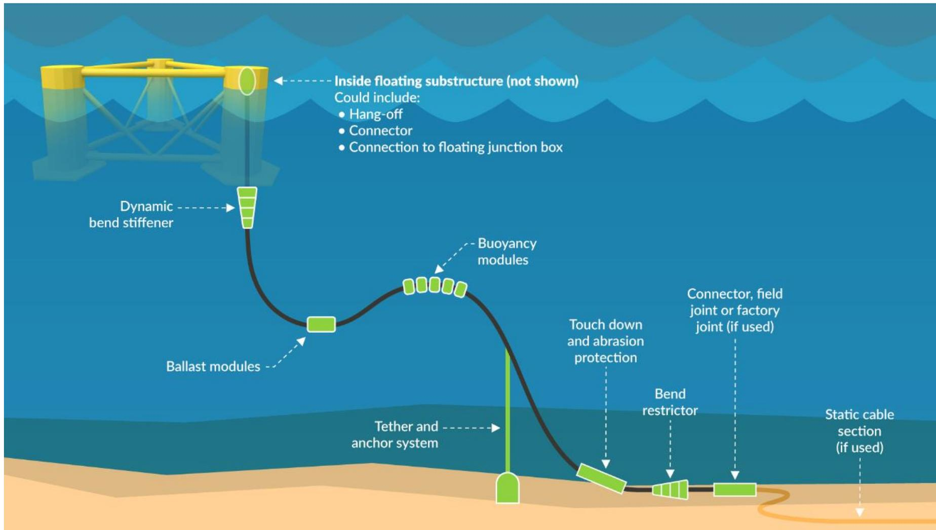
**Figure 16 Floating offshore wind dynamic cable system.** An actual system would not use all of these elements at the same time. The horizontal distance between the floating substructure and the touchdown point is typically around 200 m. *Image courtesy of BVG Associates. All rights reserved.*
