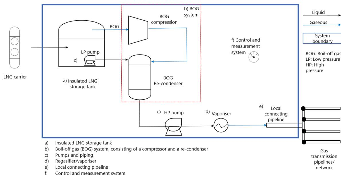
The continued risk of liquid LNG vaporising into natural gas due to heat transfer into the tank or pressure drops requires a so-called re-liquefaction system (Figure 5). It consists of a compressor and recondenser. If the boil-off gas is not removed from the tank, the pressure will increase in the tank [19]. This is only allowed for pressurized tanks.
