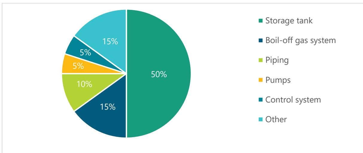
In [40], representative LNG storage tank cost are projected to lie in the range of 31-41 EUR/kg<sup>1</sup> for tanks exceeding 100 t capacity. Combining the mean value (35 EUR/kg) with the relative cost shares in Figure 3, an absolute cost distribution can be estimated, as shown in Figure 4.
