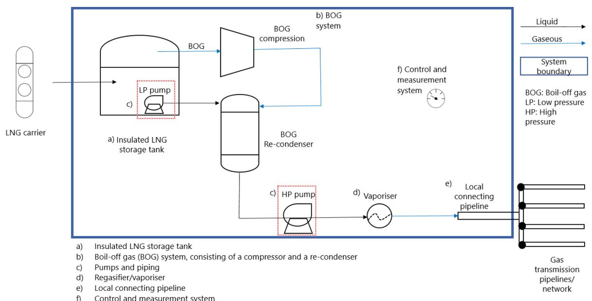
Two main pumps are used in the LNG terminal (Figure 6Figure 5). The first pump (low pressure pump) is submerged in the storage tank and pumps out LNG into the subsequent components of the terminal. The second one (high pressure pump) pumps off the liquid from the recondenser. Several other smaller pumps are located throughout the terminal.
