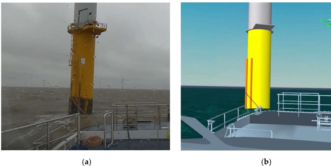
Figure 16: (a) Video footage of mooring trial in the extreme period; (b) OrcaFlex model of the same
