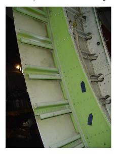
The above stringers look like they are probably extruded or rolled from sheet-metal, but the frames look like they might be candidates for structural batteries (assuming the batteries can be on their sides).
