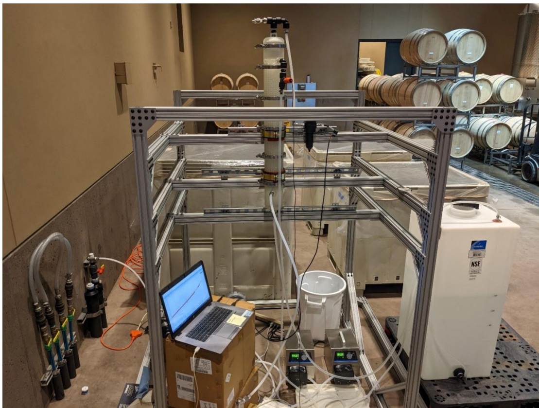
CO 2 off-gas from tanks of fermenting wine at Continuum, a Napa Valley winery, travels through plastic tubing and into the bottom of Livermore's absorber tower. Liquid solvent from the square container (right foreground) flows through the absorber packing.
