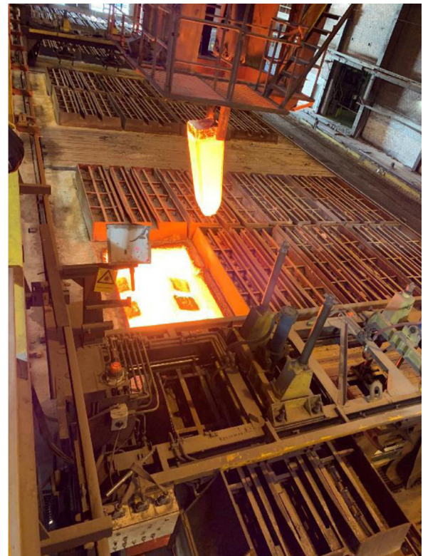
Fig. 4. Flameless oxyfuel using 100% hydrogen as fuel at world's first full-scale test of steel reheating with all hydrogen combustion in March 2020 at Ovako Steel in Sweden.
