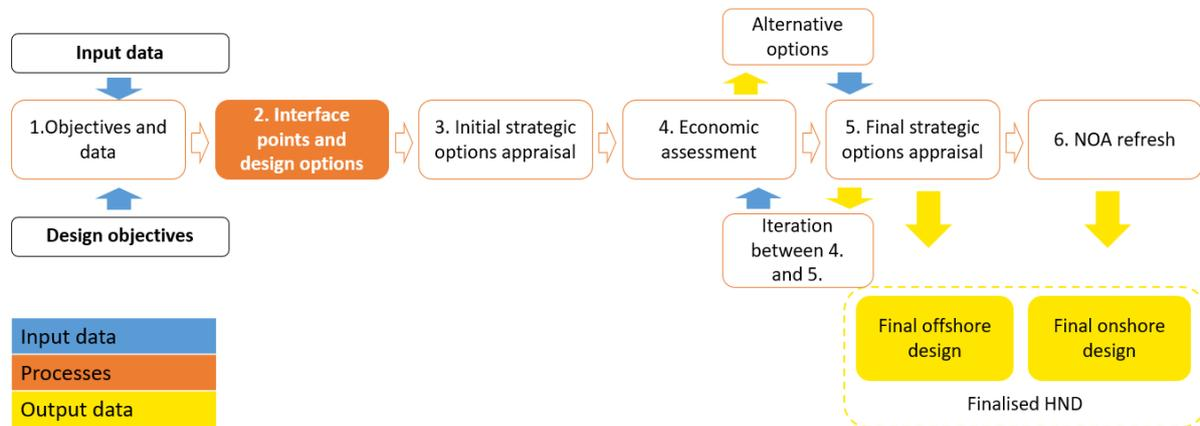
Figure 6 Step 2 - Identification of offshore design options and interface points
