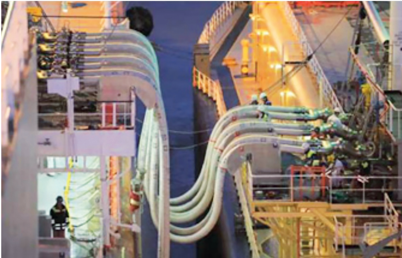
Figure 3.4 Flexible cryogenic hose system used in a side-by-side transfer configuration [Source: video still from Excelerate]
