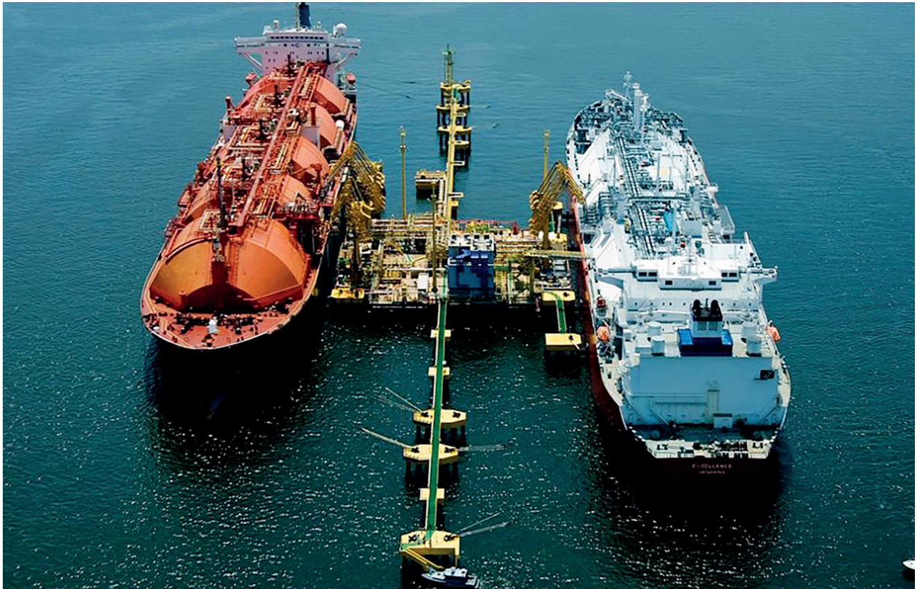
Figure 3.2 Cross-dock transfer arrangement [Source: Petrobras]
