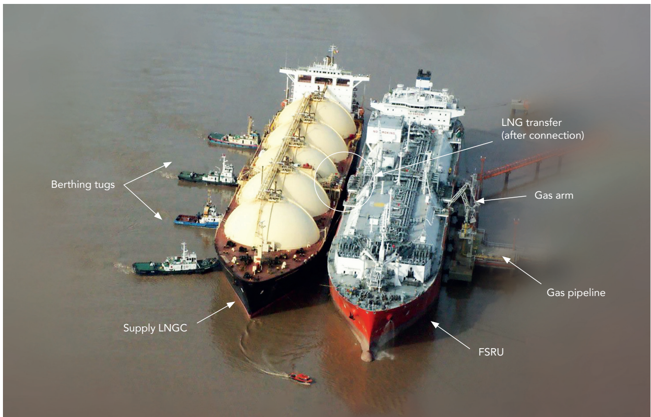
Figure 3.3 Side-by-side configurations [Source: Buques LNG]
