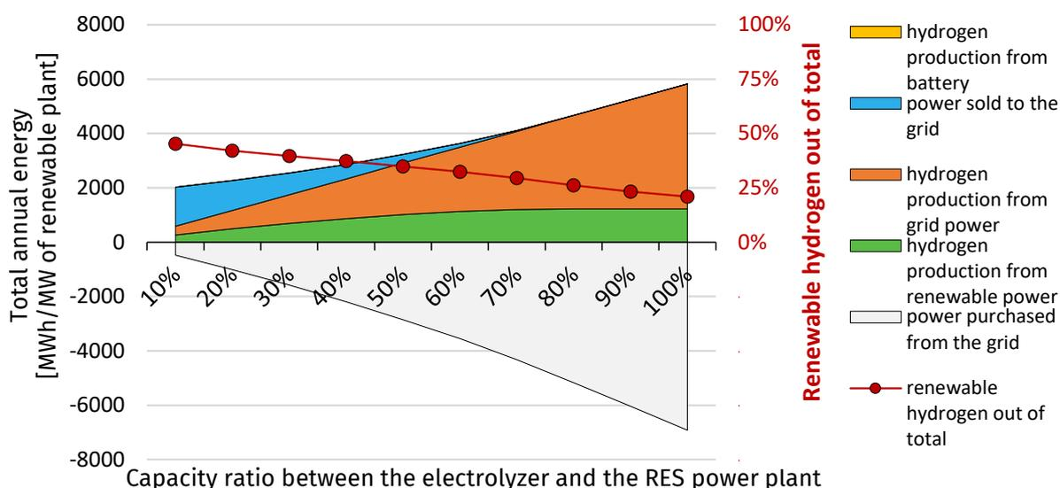
Total annual hydrogen and electricity production (left axis) and share of renewable hydrogen (right axis); case of Alexandria site, solar PV power generation, constant full-load operation of electrolyzer, without battery.
