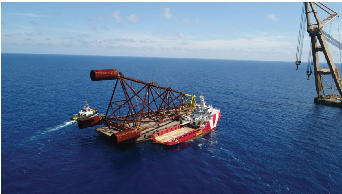
FIGURE 21.7 EXAMPLE OF JACKET FOUNDATION ON LAUNCH BARGE
